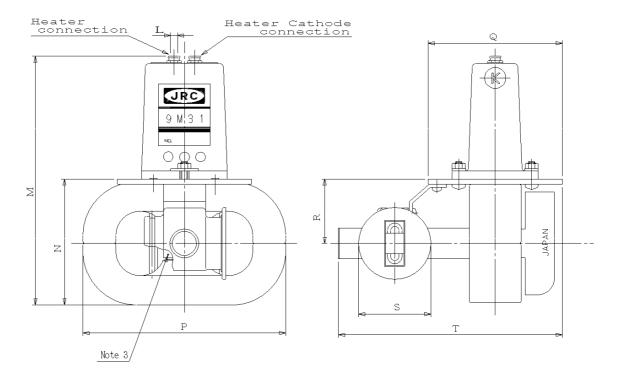
Note 3: Anode temperature measured at this point
